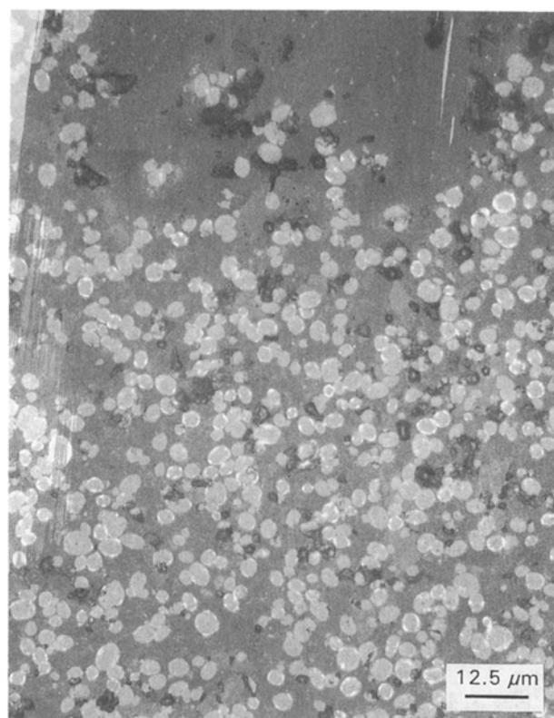
Figure 14 Scanning electron micrograph of 1550 °C sintered (CAS + ZrO 2 ) hybrid ceramic.
